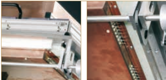
Details of RF shielding
