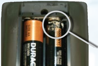
Corrosion you CAN see
