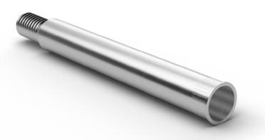
Family H348 Pitch [mm/mil] 7.60 / 300 **Electrical specifications** Continuous current [A] 100.00 Mechanical specifications Thread 5.0 Internal thread 5.0 Dimensions Total length [mm] 55.00 Press ring diameter [mm] 6.90 Outer diameter [mm] 6.50 Collar height [mm] 6.90
