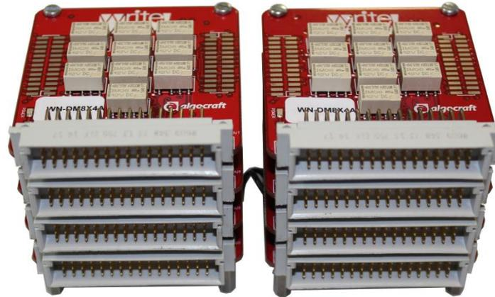
The demultiplexer module is designed to increase the number of ISP lines to be managed. A stack of up to 4 boards could be mounted to each ISP connector. It is built as a tower in order to save space. The Reed relay technology ensures true galvanic isolation and reliability.
