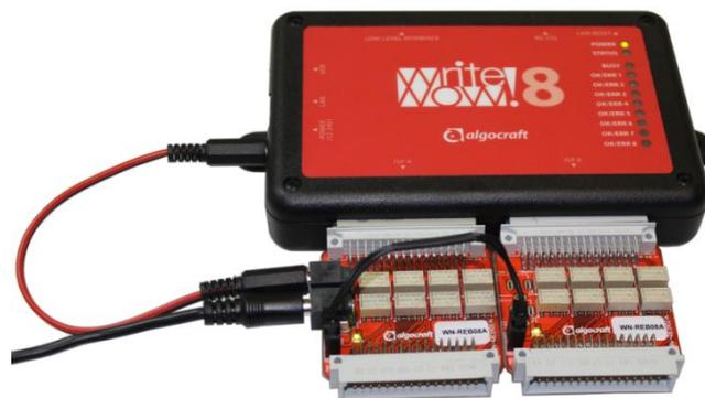
On the single-site WriteNow! model (WN-PRG01A), a relay barrier is provided on the ISP signals. On the others WriteNow! models (WN-PRG02A, WN-PRG04A and WN-PRG08A) is possible to connect externally a dedicated relay barrier module to ensure true galvanic isolation and reliability.
