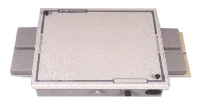
REBOUNDER® Test kits feature Two separate "Co-Active Seals", "Quick Twist" Locking Guide Pins, and boards constructed of fine weave G10/FR4, increasing testing reliability and accuracy while simplifying finishing, debugging and maintenance. All H+W Products are backed - up with our "Test-Assured" one year warranty -- In Writing -- and SAME DAY SHIPMENTS.
